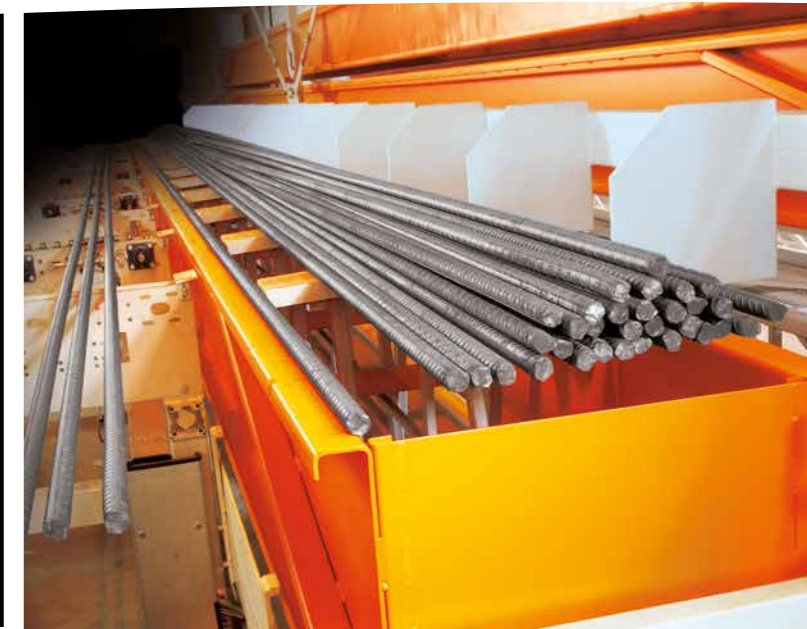
Longitudinal chain conveyor with lift unit.
