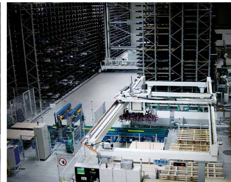
Honeycomb storage system for bar stock/sheet metal with fully automatic sheet metal picking system
