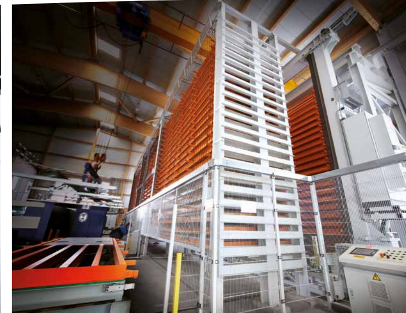
Storage of sheet metal packages and retrieval station for manual loading of a laser cutting machine.
