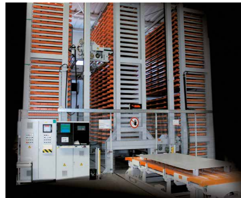
UNITOWER B extended to two operating gantry cranes.
