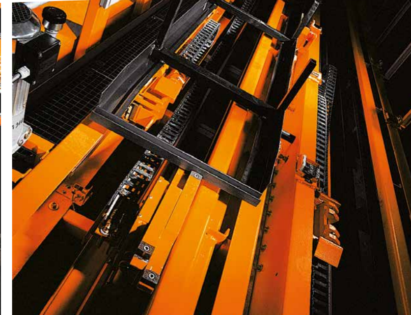
Operating gantry crane with towing device for reliable cassette transport. UNIGRIP longitudinal chain conveyor: for easy storage and removal at the front of the shelf.
