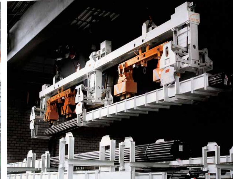
UNIBLOC F with combination traverse for transporting cradles and removing rods.
