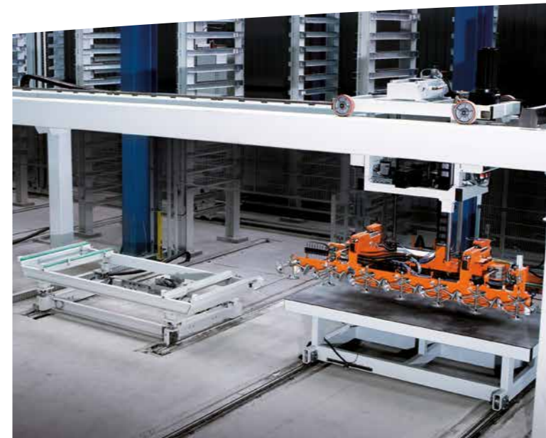
Automatic picking station with vacuum transport system.
