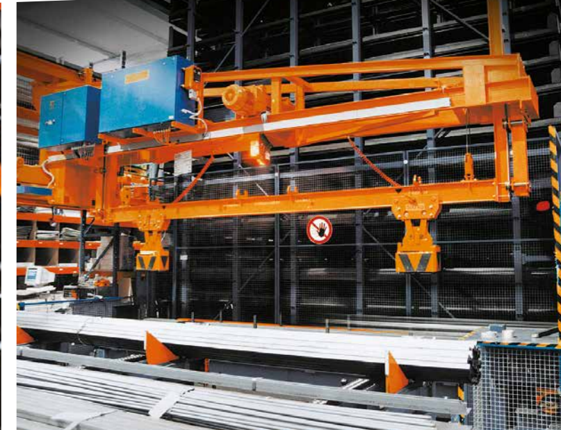
The picking device allows for an ergonomic and fast material removal.
