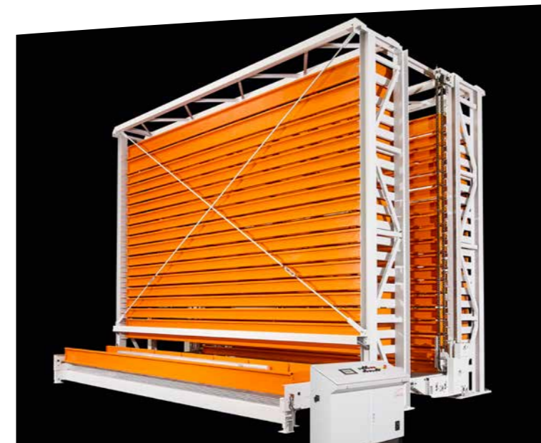
Bar stock variant in double-sided design (option).
